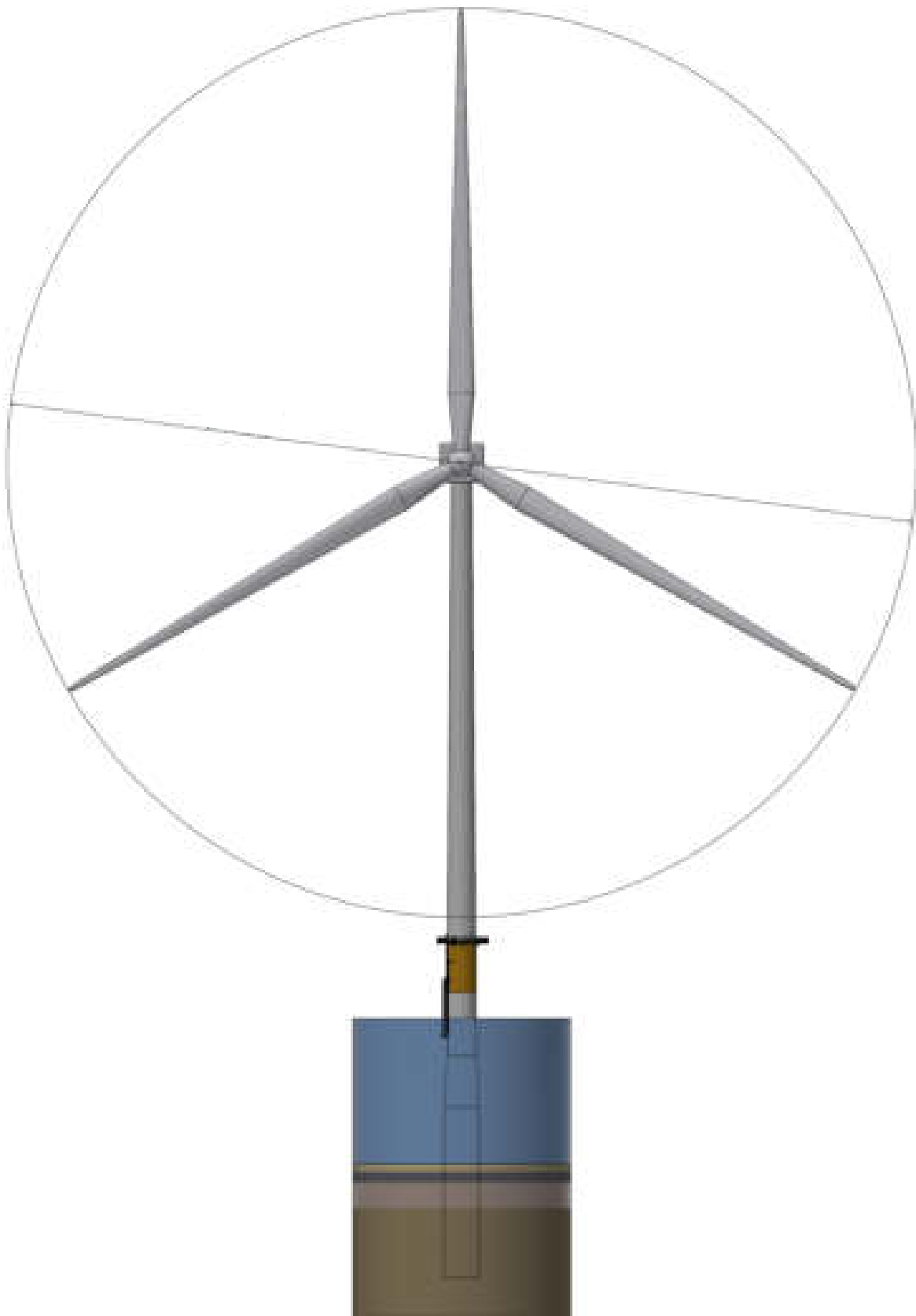
Figure 3: Monopile general arrangement for Site 1 C4 -40mWD, diameter up to 9.5 m
