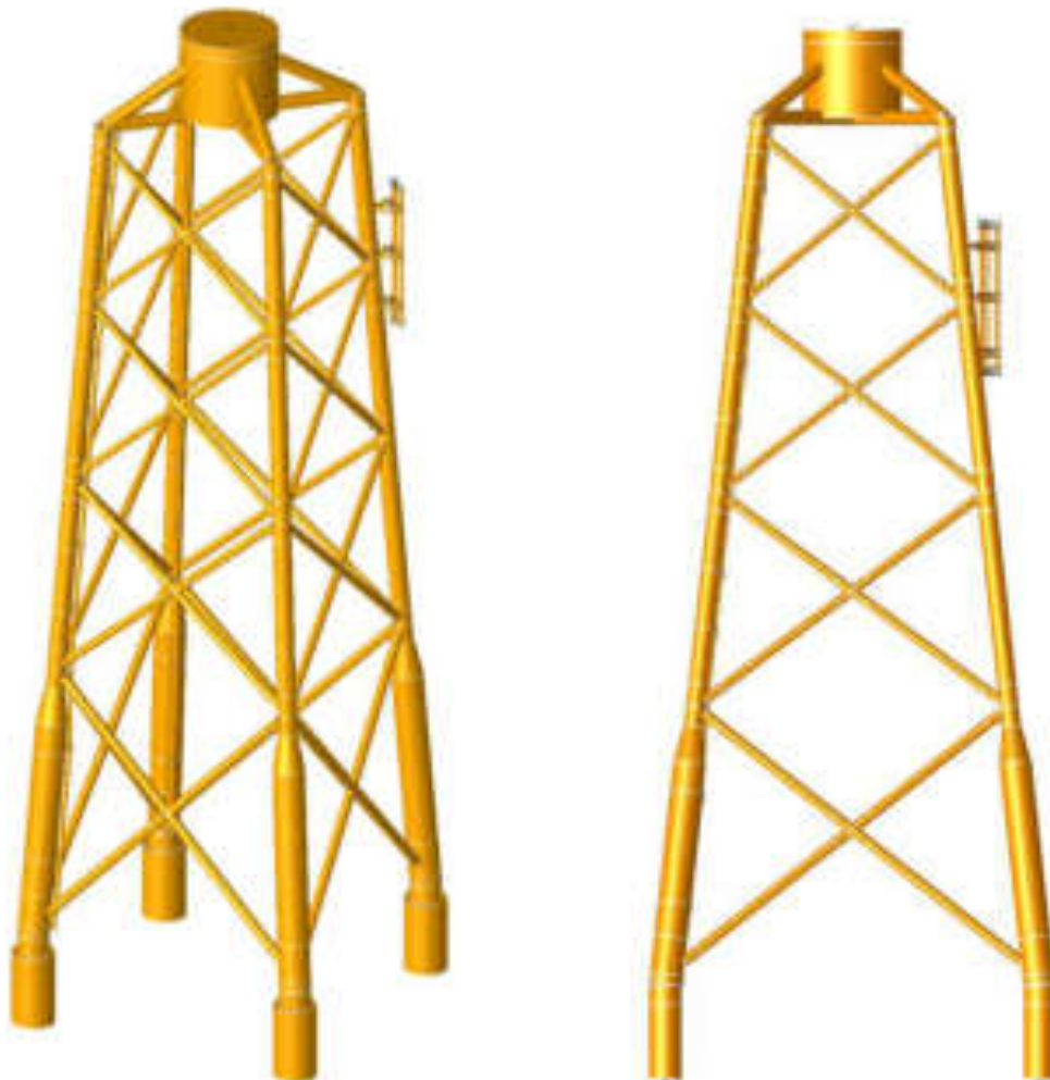
Figure 3-14: Jacket Site 3 (60 m water depth), left: 23.25m FP, right: 30m FP
