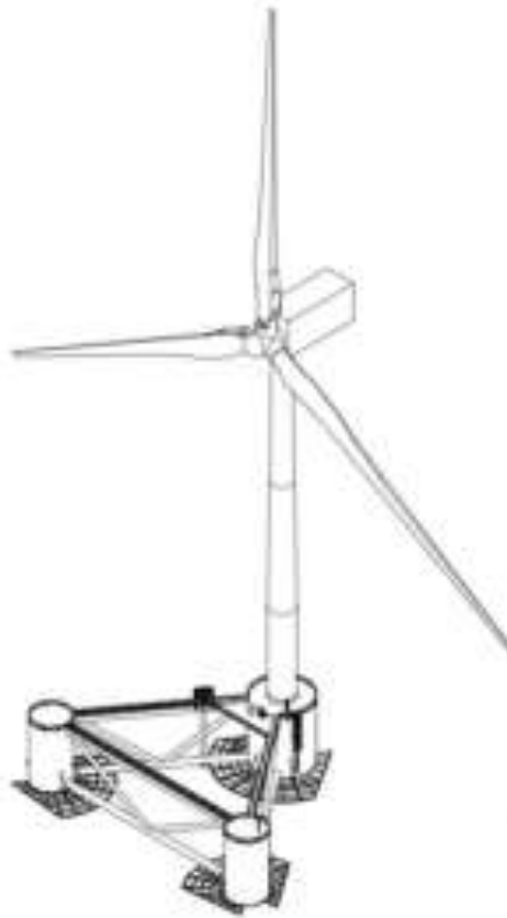
Figure 21: A generic conventional WindFloat-T with a wind turbine
