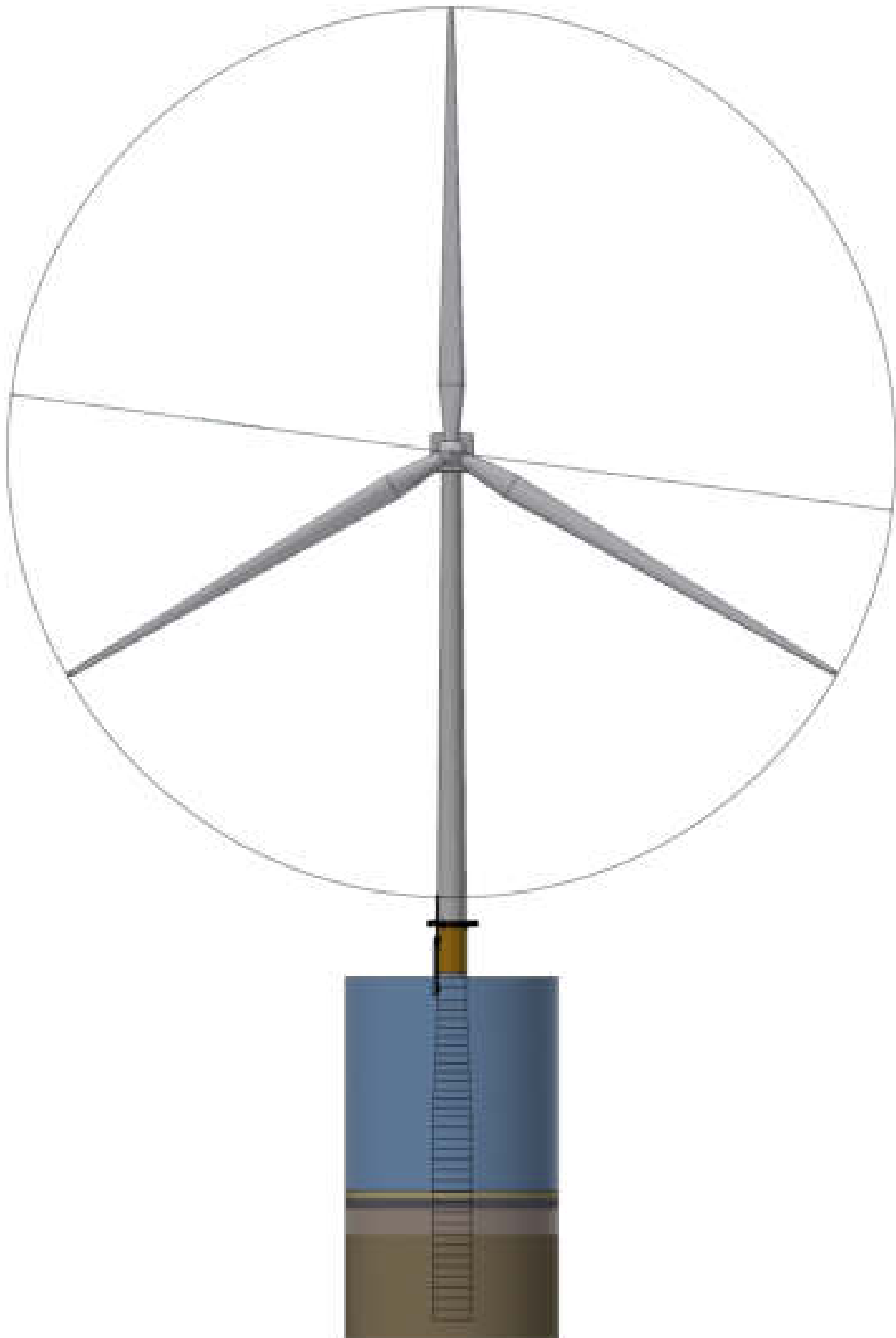
Figure 7: Monopile general arrangement for Site 3, -60mWD, diameter up to 11.0 m
